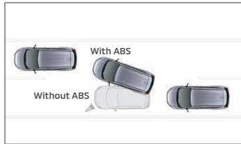
ABS (Anti-lock Braking System), EBD (Electronic Brake Distribution) with Brake Assist (BA)
